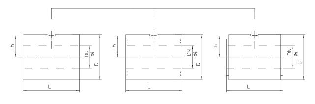
flange connection per DIN or ASME plain raised face nominal pressure max. 400bar flange connection per DIN with nut, model D nominal pressure max. 10-100bar flange connection per DIN with projection, model D nominal pressure max. 10-100bar
