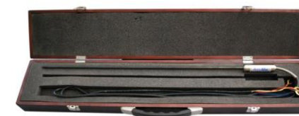
AccuMac 1860-25 Range: -200°C to 670°C Standard platinum Resistance thermometer
