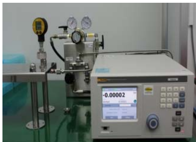
Fluke Controller PPC4EX-7M 7MPa & 700kPa / 0.005% of F.S
