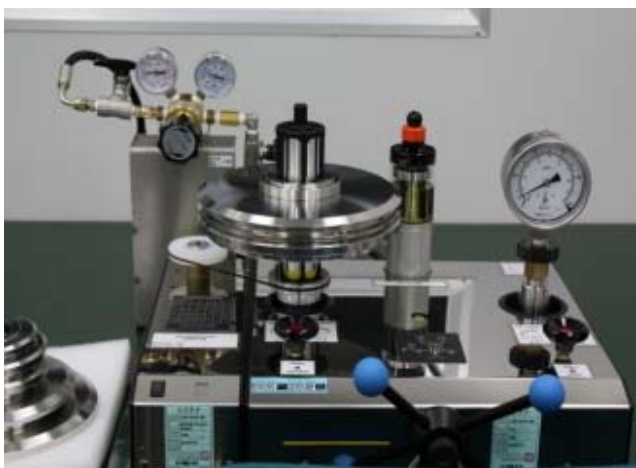
Europascal Pneumatic DWT-BA2-70 Max. 70bar / 0.007% of rdg.
