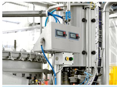
Figure 2 Gas sampling application with two gas flow meters
